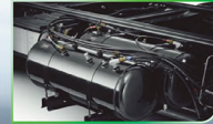
Phanh khí nén toàn phần (FVR/FVM/FVZ) Full-air brake with air dryer (FVR/FVM/FVZ)
